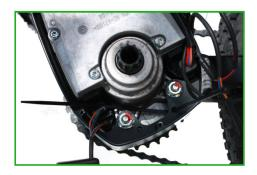
**6.** Fasten the bikespeed-RS at the shown position using the cable binder.
