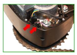
Remove the cable binder and move the original cables you just removed to the gap between motor and frame.
