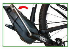
Remove the five screws of the gravel deflector and then remove it. Use a Torx T20 for untightening the screws.
