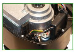
Connect the two removed connectors of the original cables with the white sockets on the bikespeed-RS. The plugs are coded and can only be plugged in the correct direction. Please do not use force!
