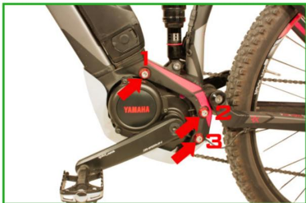
**2. It is possible that your motor is attached to more screws of further covers. These must be removed as well. (See example, one screw on the left and right of each arrow):**
