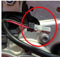
6. Put the plug of the bikespeed-cable set into the socket that has become available.
