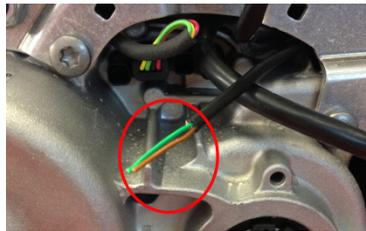
9. Skin the brown and grey conductor of the bikespeed- cable set (USB-slot) by about 5mm.
