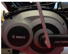
2. Dismount the treadle with a suitable crank puller (e.g. picture: Lifu, used for most bicycles with a Bosch-engine)
