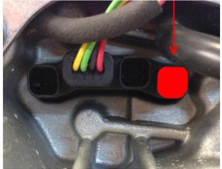
The removed plug is two-pole and grey.
