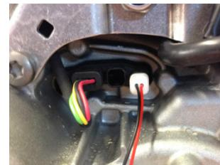
The plug has to be inserted as far as it will go. The silicon seal may no longer be visible. Upon delivery we apply some Vaseline onto the seals for lubrication. If there is not enough lubrication, you may renew it. Please advance with care when you insert the plug. Do not use force!
