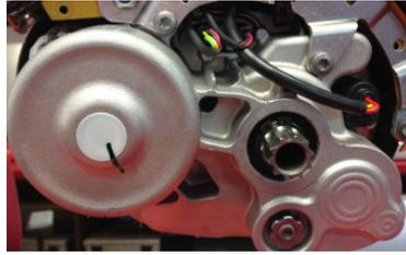
5. Remove the plug of the speed sensor.
