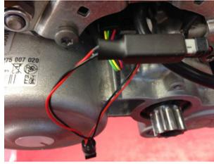
Also put the plug so far into the socket that the seal is no longer visible.
