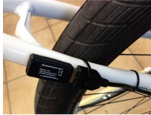
Carry the cable to the area of the gravel deflector. The cable of the bikespeed-key cable set can be shortened to the length required.
