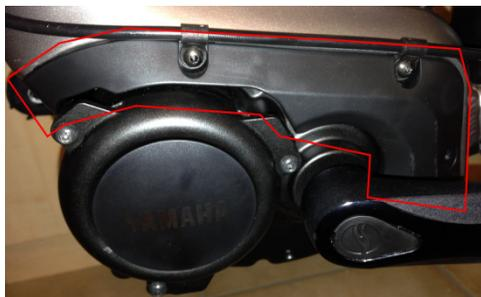
3. It is possible that your engine is attached to more screws of further covers. These have to be removed as well.
