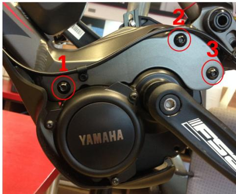
2. You possibly have to remove a plastic cover in order to get to the fastening screws of the engine.
