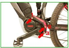
2. It is possible that your motor is attached to more screws of further covers. These must be removed as well. (See example, one screw on the left and right of each arrow):
