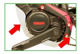
When the motor is folded down, expose the two connectors to the display (4-pole, white) and the speed sensor (3-pole, white) and unplug them. Therefore, please press the retaining tabs at the arrow-marked sites.
