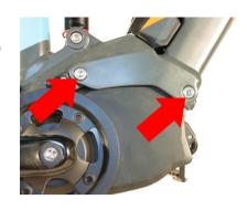
2. On the left, loosen the screw (1) shown on the left with a 6-inch Allen key. The screw remains in place and serves as a hinge for the engine to be folded down (2).
